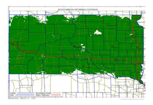
Over the course of the past 9 years, an additional 19 sites have been installed, and over 8,000 radios have been added to the network. The current system has 54 sites on line, 304 voice repeaters, and now exceeds 98% of the geography of the state. (See below map)
