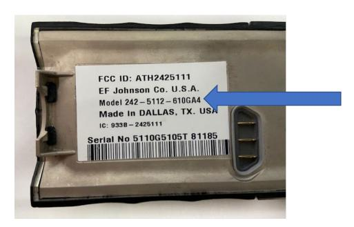
The above arrow identifies where to locate model information after battery removal.
