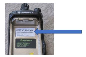
The above arrow indicates where to find the Flashcode on portable radios after removing battery.
